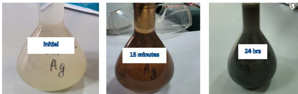
Figure 1. Color intensity after the addition of algal cell-free extract with 1 mM \text{AgNO}_3 , indicates formation of silver nanoparticles. a) initial color change, (b) 15 minutes, (c) 24 hrs.
