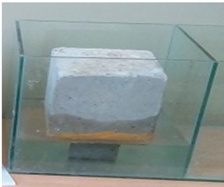
Fig. 14. Concrete Specimen Sorptivity test
